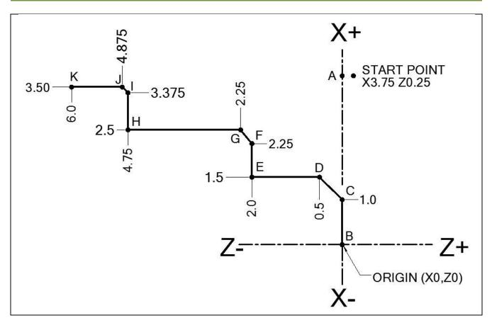
BEGIN AT START POINT SP (X3.75, Z0.25), DESCRIBE THE PATH FROM SP THROUGH POINTS A-K AND BACK TO POINT SP, USING ABSOLUTE & INCREMENTAL POSITIONING
