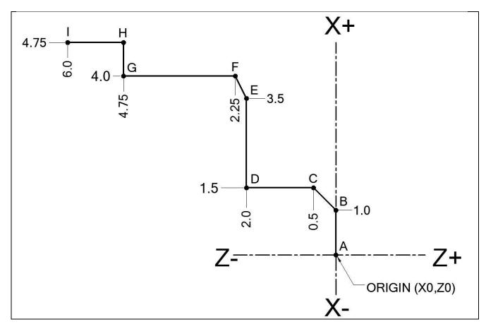
STARTING AT THE POINT A (ORIGIN), DESCRIBE THE TOOLPATH THROUGH ALL THE POINTS USING ABSOLUTE & INCREMENTAL POSITIONING
